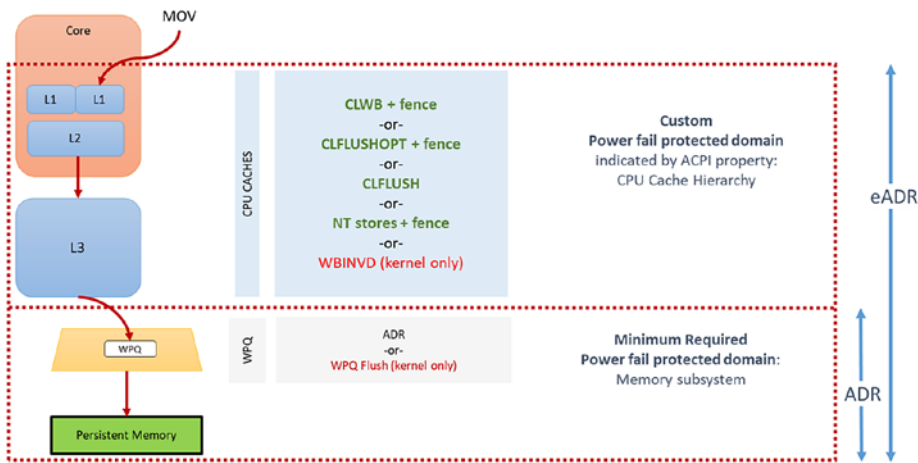
Figure 2-2. ADR and eADR power-fail protection domains
