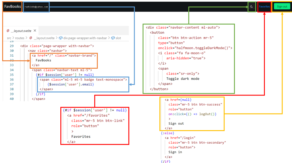
Figure 5-i: Main Page UI and Markup ( __layout.svelte ) Relationship (Just Considering the Navigation Bar)
