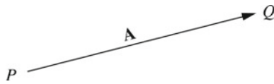
Fig. 1.1 A vector is represented geometrically by an arrow PQ 129 drawn to scale
